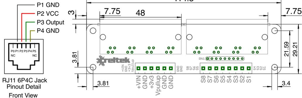
All dimensions in millimeters. Tolerance  $\pm 0.5$  mm.
